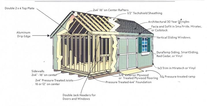
Sub Foundation: Pressure treated 4x4s 30 yr. (3 to 5 depending on building width)
