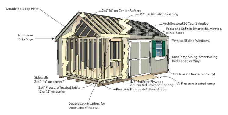
Sub Foundation: Pressure treated 4x4s 30 yr. (3 to 5 depending on building width)
